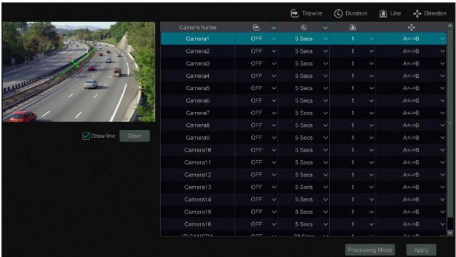
② Select the camera, enable the line crossing detection and set the duration.
