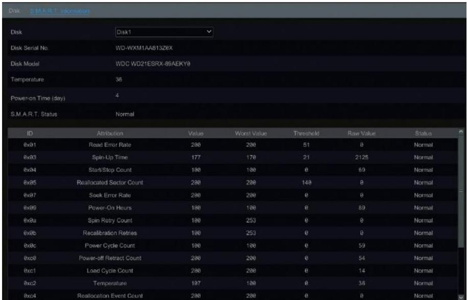
The screenshot shows the S.M.A.R.T. Information interface for Disk1. The interface includes a dropdown menu for the disk name, and several fields for disk details: Disk Serial No., Disk Model, Temperature, Power-on Time (day), and S.M.A.R.T. Status. Below these fields is a table of SMART attributes.
