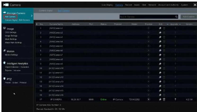
There are some function items on the left side of the camera management interface. Click each item to go to corresponding interface or window. For instance, click “Add Camera” to pop up the window as shown below.
