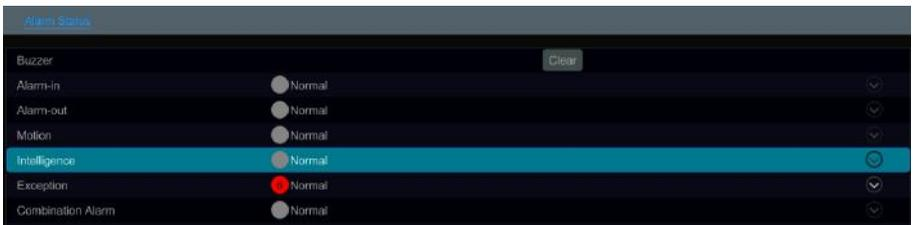
Click the “Clear” button to stop the buzzer when the buzzer alarm happens. Click
