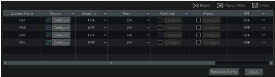
② Enable or disable “Record”, “Snapshot”, “Push”, “Alarm-out”, “Preset”, “Buzzer”, “Pop-up Video” and “E-mail”. The alarm handling setting of exception detection alarm is similar to that of the sensor alarm (see [9.1 Sensor Alarm](#) for details).
