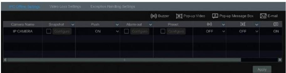
② Enable or disable “Snapshot”, “Push”, “Alarm-out”, “Preset”, “Buzzer”, “Pop-up Video”, “Pop-up Message Box” and “E-mail”. The IPC Offline Settings are similar to that of the sensor alarm (see [9.1 Sensor Alarm](#) for details).
