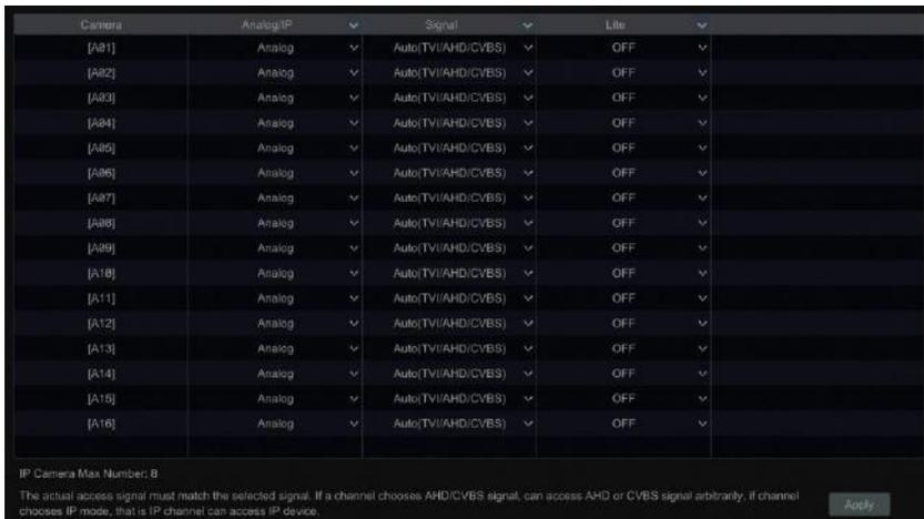
**Note:** You can enable “Lite” in the interface if the DVR supports “Lite” recording. It will lower the recording resolution and increase the recording frame rate. Please enable or disable the Lite as needed.
