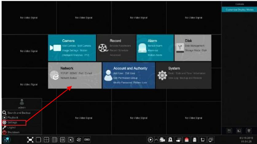
The setup panel includes seven modules. Each module provides some function entries with links for convenient operation.
