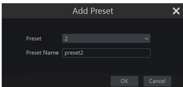
Adjust the dome’s direction and then click “Save Position” to save the current preset position (you can also click another preset in the preset list and then save the preset position after adjusting the dome’s direction); click
