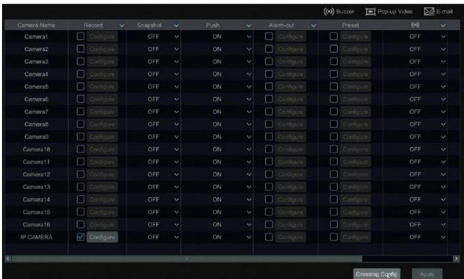
② Enable or disable “Record”, “Snapshot”, “Push”, “Alarm-out”, “Preset”, “Buzzer”, “Pop-up Video” and “E-mail”. The alarm handling setting of line crossing alarm is similar to that of the sensor alarm (see [9.1 Sensor Alarm](#) for details).
