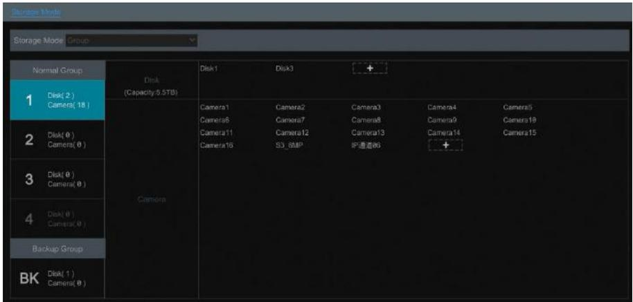
There are four disk groups. By using disk group, you can correspond the camera to disk (the record data of the camera in the group will be stored into the disks in the same group). The DVR with e-SATA interface supports e-SATA recording.
