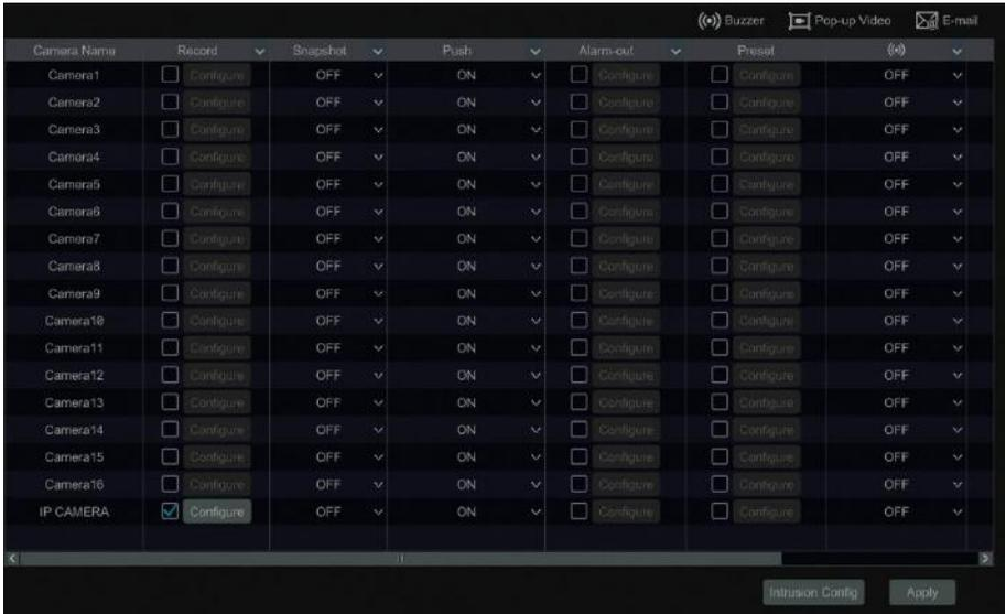
② Enable or disable “Record”, “Snapshot”, “Push”, “Alarm-out”, “Preset”, “Buzzer”, “Pop-up Video” and “E-mail”. The alarm handling setting of intrusion detection alarm is similar to that of the sensor alarm (see [9.1 Sensor Alarm](#) for details).
