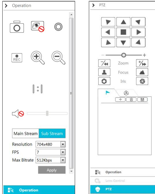
Click one camera window in the preview area and then click Main Stream to set the camera's live preview stream and record stream to main stream in manual record mode; click Sub-stream to set the camera's live preview stream and record stream to sub stream. In sub stream tab, set the resolution, FPS and bitrate and then click "Apply" to save the settings.
