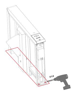
6. Clean up the soil and dust after the drilling is completed, place the turnstile to the installation site again.
