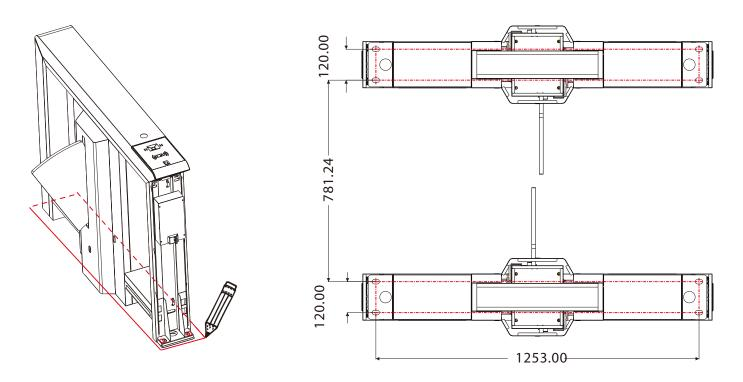
5. Take the turnstile aside and use the electric drill according to the drawn screw holes.
