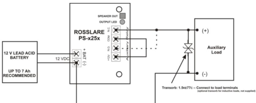
Figure 4 shows the auxiliary output connection using the external power.
