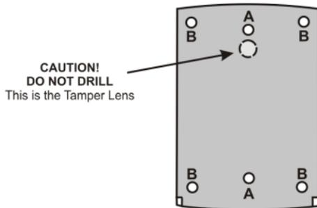
5. Drill a 10-mm (7/16") hole for the cable. If the surface is metal, place a grommet or electrical tape around the edge of the hole.
