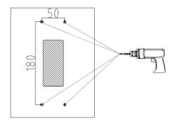
As figure shown, mark four screw holes on the position that according to the cable place. The horizontal distance of two holes should be 50 mm, and the vertical distance of two holes should be 180 mm. Then use a hand drill with a diameter of 6 mm to drill the four marked holes with a depth of 20 mm.
