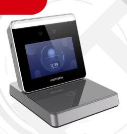
The enrollment station can realize multiple user information's enrollment on one device. It supports enrolling face picture, 13.56 MHz IC card No., and 125KHz ID card No.
