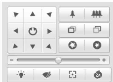
Figure 4-4 PTZ Control Panel
