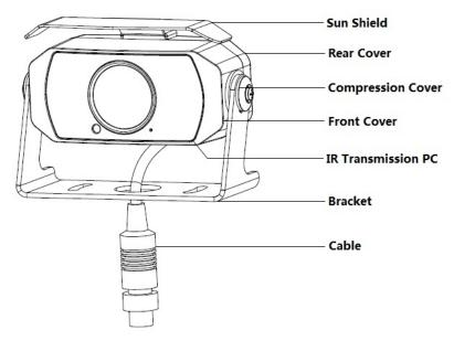
Figure 2-7 See Figure 2-8 for the cable sequence of **model C**.
