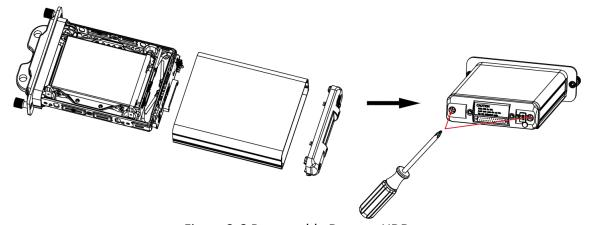
Figure 2-6 Reassemble Dummy HDD
