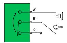
Figure 2-13 Alarm Output Connection
