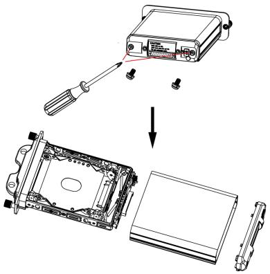
Figure 2-2 Take Apart Dummy HDD
