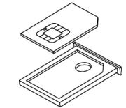
Figure 2-9 Place SIM card on SIM Card Tray
