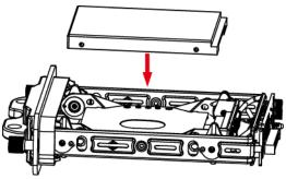
Figure 2-3 Place HDD
