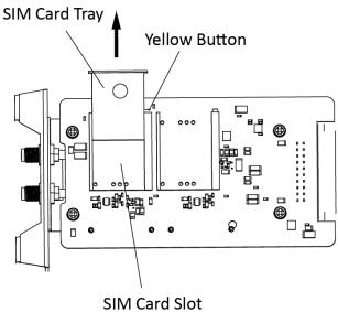
Figure 2-8 Pull out SIM Card Tray
