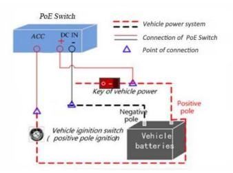
Figure 2-14 Connection of Positive Pole Ignition Switch
