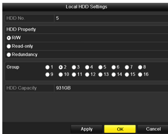
Figure 14-13 Local HDD Settings Interface
