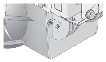
b. Attach a ground wire (min. 8 AWG or 10 mm²) to the lug and replace the nut to secure the wire.
