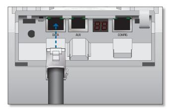
Connect the other end of the Ethernet cable from the DATA port to the Ethernet port labeled POE on the PoE Adapter.
