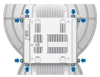
WARNING: Before you begin the alignment process, all Lock Bolts MUST be loose to avoid damage to the airFiber housing.
