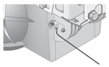
c. Secure the other end of the ground wire to the pole, tower, or grounding bar.
