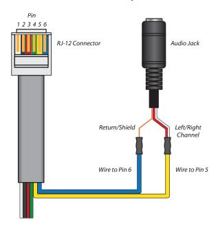
Pinouts from RJ-12 to 3.5 mm Stereo Phono Jack
