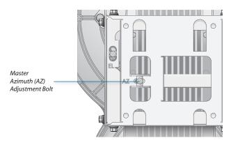
b. Sweep the *Elevation (EL) Adjustment Bolt* of the *Master* through its adjustment range.
