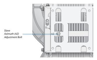
b. Sweep the *Elevation (EL) Adjustment Bolt* of the *Slave* through its adjustment range.
