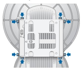
4. Secure the four M8x16 Serrated Flange Screws to the back of the Alignment Bracket. Do not completely tighten the screws; leave a 6 mm gap between each screw head and the bracket.
