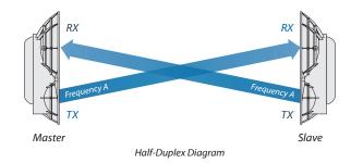
For Full Duplex mode, the TX and RX Frequencies should be different.
