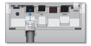
3. Create a strain relief for the Ethernet cable by feeding a cable tie through the tie slot under the cable. Then wrap the cable tie around the cable and tighten.
