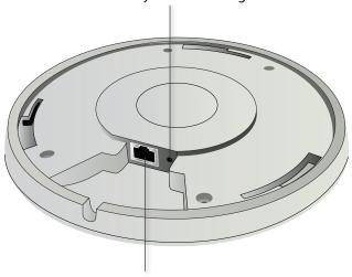
**Ethernet Port** Connects to the 24v PoE Adapter to provide power to the unit.
