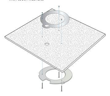
Feed the Ethernet cable through the hole and then align the UniFi AP with the notches on the wall-mount bracket.
