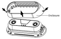
Figure 2-10 Remove the Enclosure
