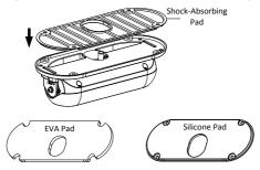
Figure 2-11 Attach Shock-Absorbing Pad
