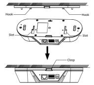
Figure 2-3 Install the Camera
