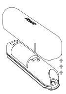
2. Remove the battery blocker.
