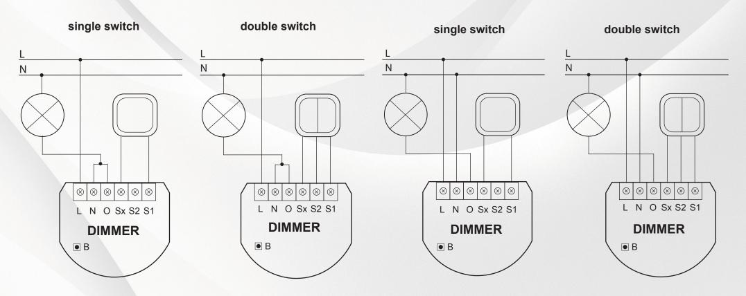
Electrical diagram for connecting the Dimmer - 2-wire connection
