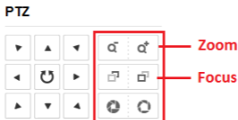
Figure 2-17 Zoom and Focus Adjustment via Web Browser
