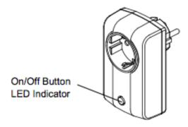
The electrical load can be switching using wireless commands and operating the local button. The LED inside the local button will indicate the switching status.
