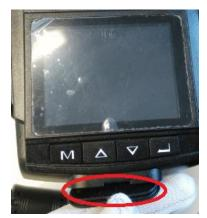
Figure 3-1 Open Cover of SIM Card Slot
