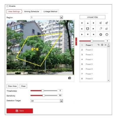
Figure 5-23 Configuring Intrusion Area
