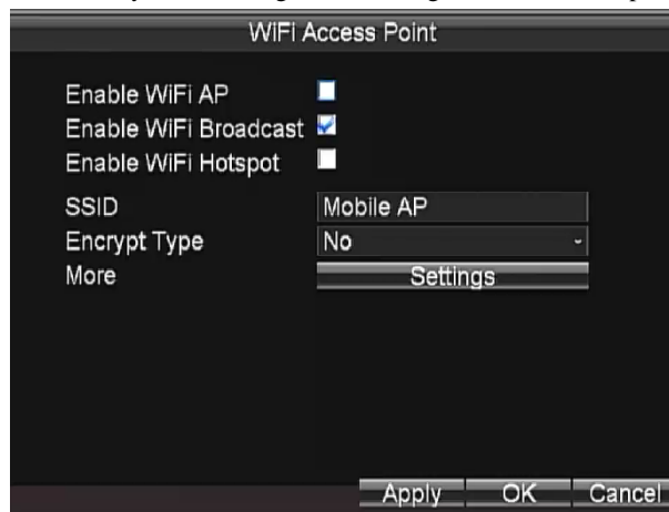
Figure 5. 5 Wi-Fi Access Point Settings
