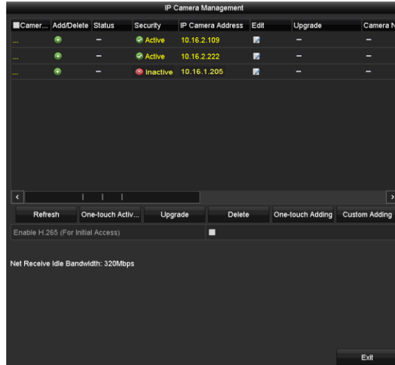
Figure 2-36 IP Camera Management Interface
